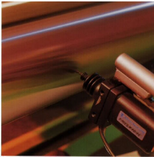
A probe registers shape and concentricity
