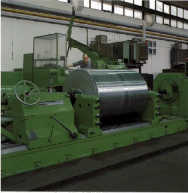
Cooling roll on the grinding machine
